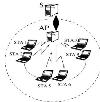
Figure 1: IEEE 802.11 DCF based WLAN Access Scenario
