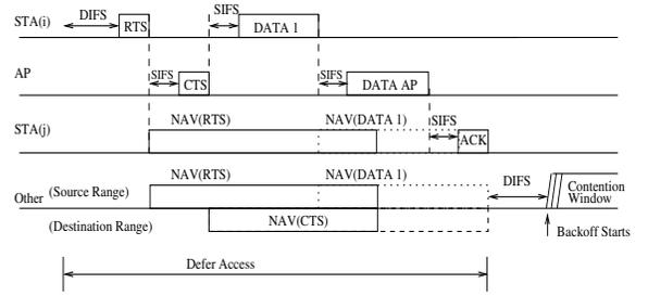
Figure 3. Timing diagram of BDCF with RTS-CTS handshake
