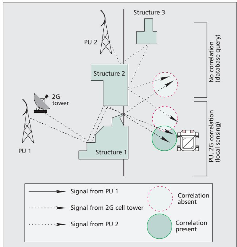
**Figure 2.** Illustration of the PU and 2G signal correlation that occurs at selected locations in the CRV's path.
