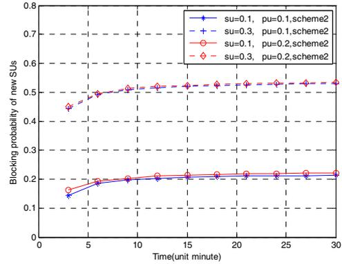
Figure 8. The blocking probability of new SUs in scheme 2 when both  $\lambda_{PU}$  and  $\lambda_{SU}$  change
