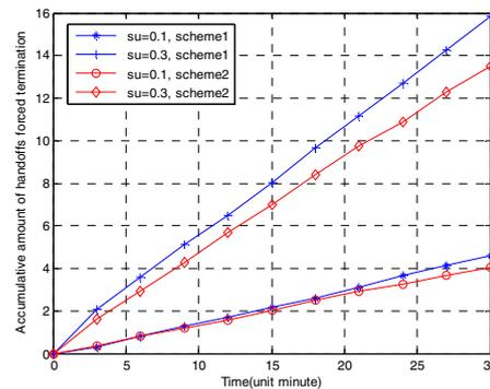
Figure 4. The accumulative amount of handoffs forced termination for SUs when  $\lambda_{PU}=0.1$
