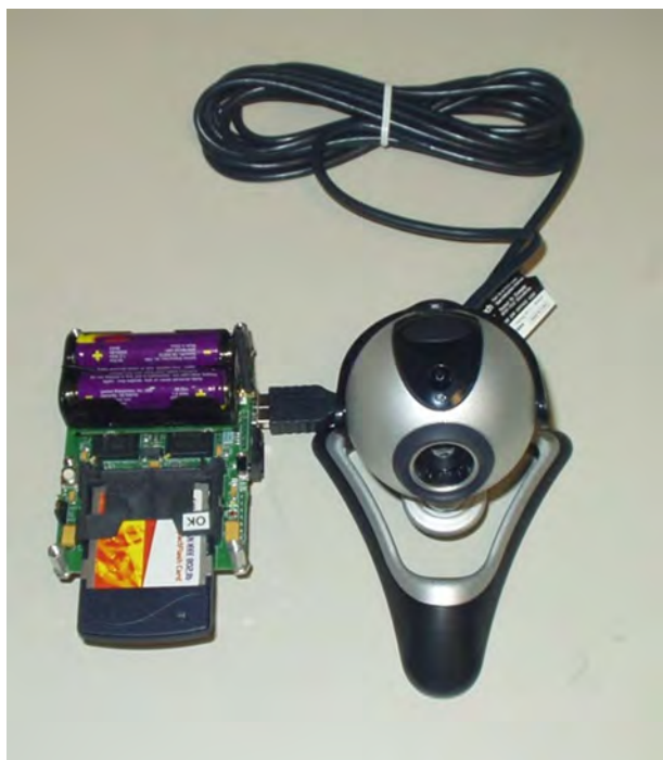
Fig. 7. Stargate board interfaced with a medium resolution camera. Stargate hosts an 802.11 card and a MICAz mote that functions as a gateway to the sensor network.
