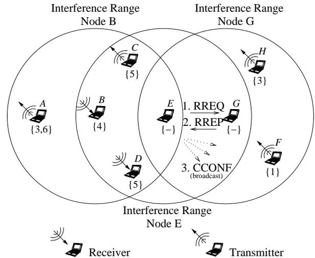
**Figure 1: RREQ coverage area and formation of favorable sets at the transmitter and receiver. The channels used by an MR are indicated in the parenthesis.**
