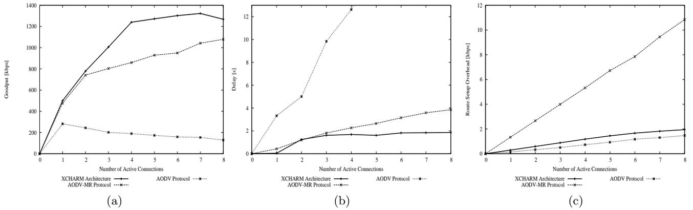
Figure 3: Channel Selection Analysis, Variable Number of Active Connections: (a) End-to-End Goodput, (b) End-to-End Delay, (c) Route Setup Overhead Rate
