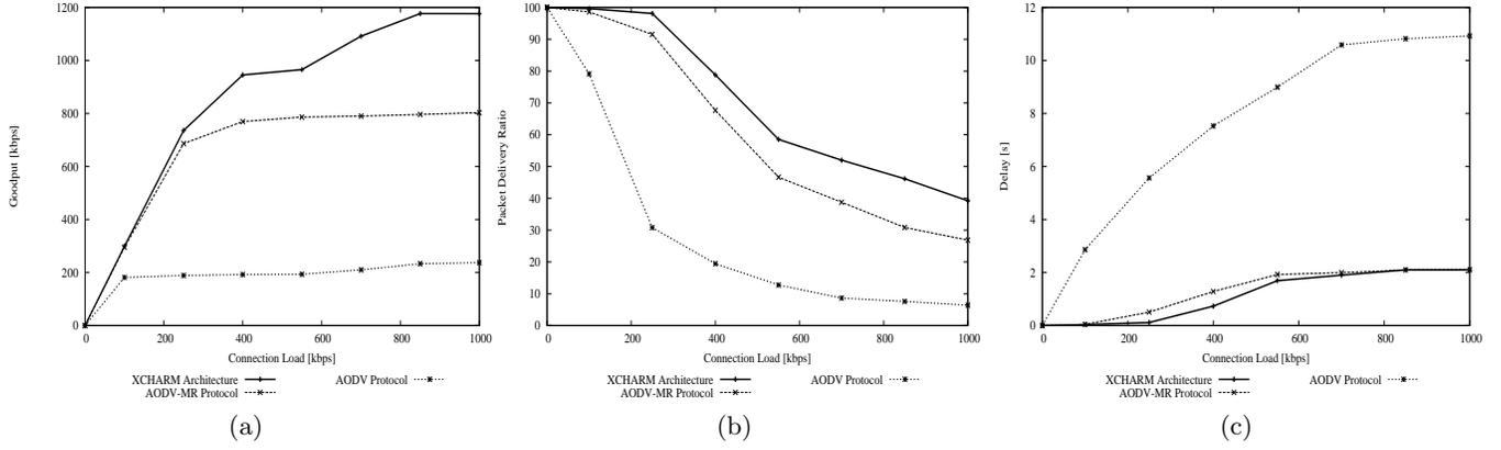
Figure 2: Channel Selection Analysis, Variable Connection Rate: (a) End-to-End Goodput, (b) Packet Delivery Ratio (PDR), (c) End-to-End Delay
