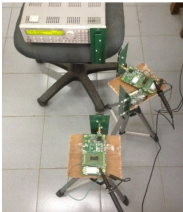
Figure 1. Experimental setup of two-hop energy transfer.
