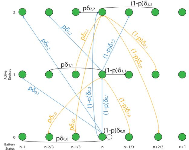
Fig. 1.  $(M+1)kN$  states model,  $M=2$  and  $k=3$  centered at state  $n$
