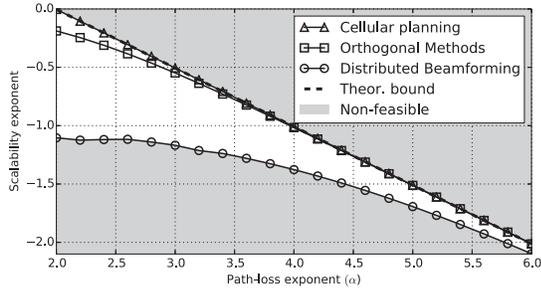
Fig. 3. Design space of multiple access methods for Multi-ETs in terms of the scalability of the minimum cumulative injected power as a function of the path-loss exponent.
