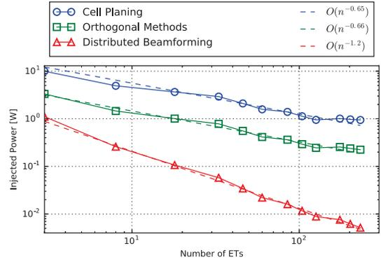
Fig. 2. Minimum cumulative power injected by the ETs to guarantee sufficient harvested power at any location, considering a regular hexagon deployment grid.
