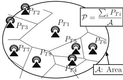
Fig. 1. Voronoi tessellation generated by the energy transmitters and graphical definition of the cumulative injected power density.
