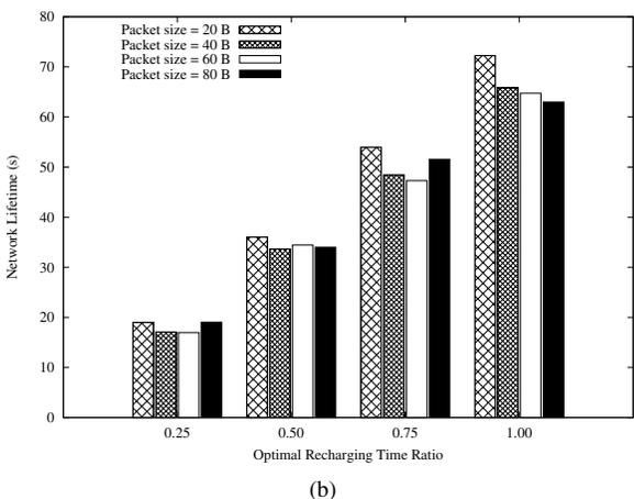
Fig. 4. The end-to-end throughput (a) and the network lifetime (b) for different packet sizes measured against increasing charging time ratio.
