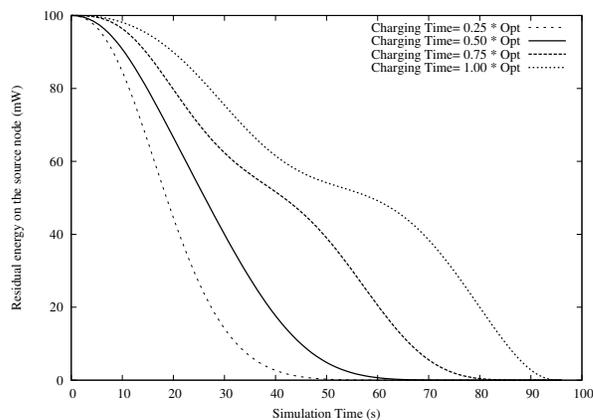
Fig. 5. Residual energy at the source node as function of simulation time.
