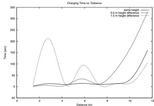
Fig. 2. Variation of the charging time of a capacitor on the receiver as function of increasing distance for different transmitter-receiver heights.
